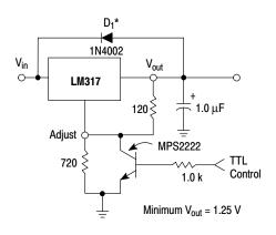
\*  $D_1$  protects the device during an input short circuit.
