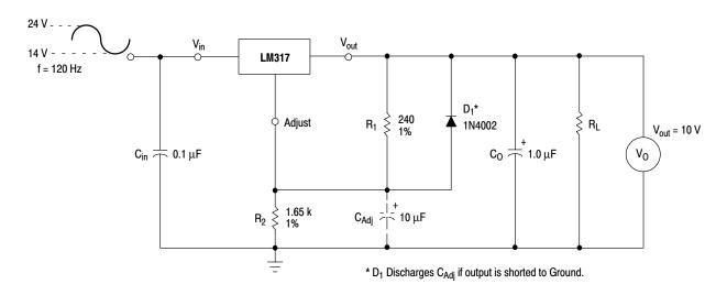
Figure 6. Ripple Rejection Test Circuit
