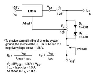
Figure 23. Adjustable Current Limiter
