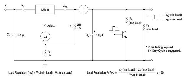
Figure 4. Load Regulation and  ${\bigtriangleup I}_{\text{Adj}}\text{/Load}$  Test Circuit
