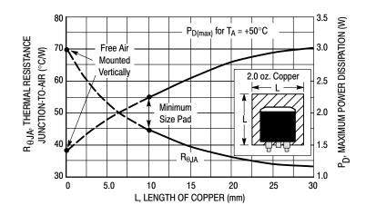
Figure 21. D<sup>2</sup>PAK Thermal Resistance and Maximum Power Dissipation versus P.C.B. Copper Length
